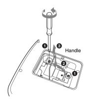
5 Insert the new lamp all the way in until it is securely in place (1). Tighten the two screws (2). Fold down the handle to replace it (3).
