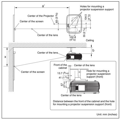
This section describes the examples for installing the projector on the ceiling.
